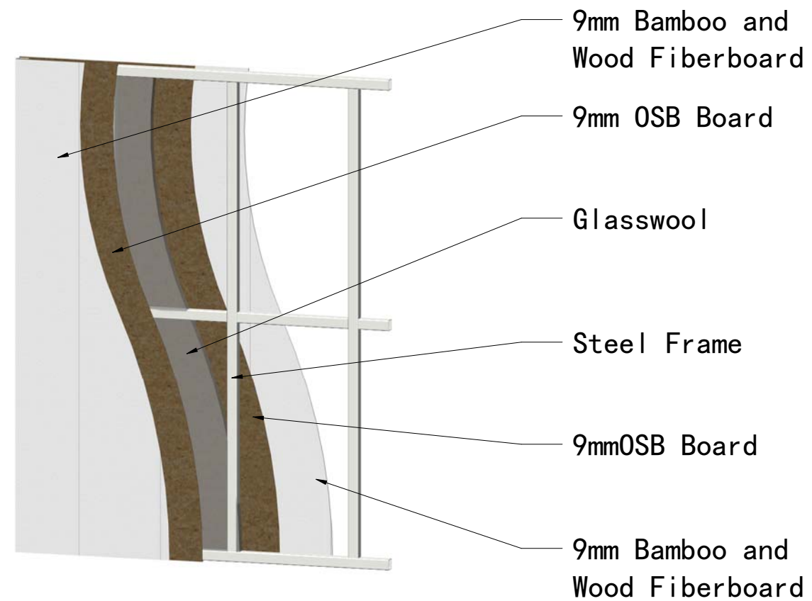
Section View of Interior Wallboard
